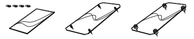
Additional Shelf (full size) (hwd 6 x 550 x 330) Isolation Platform (full size) (hwd 40 x 720 x 420) Floor Isolation Slab (full size) (hwd 90 x 720 x 420)
